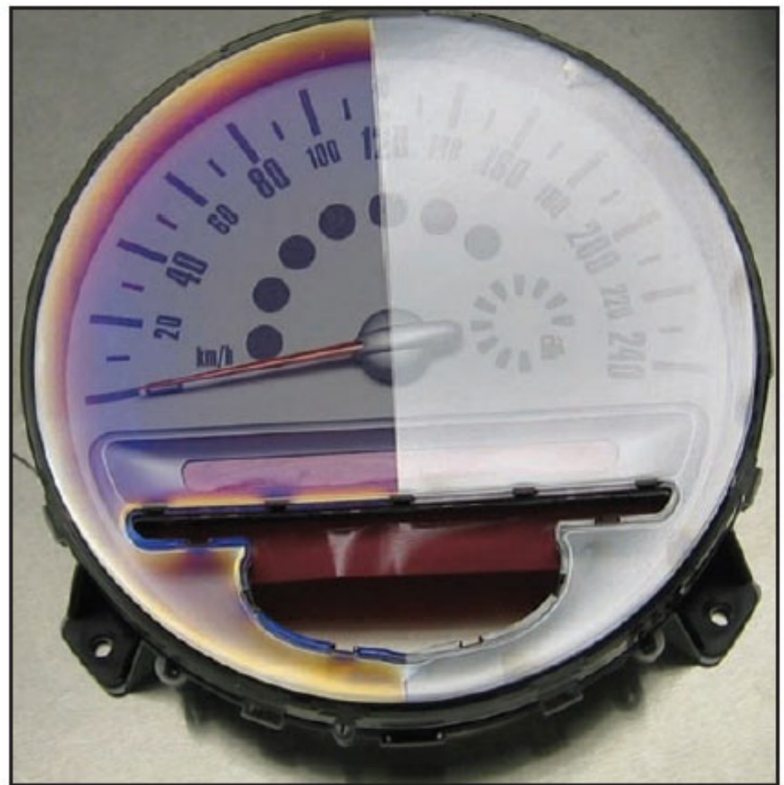
Figure 2. A high-performance antireflection coating has been deposited on one side of this plastic automotive instrument display window.
