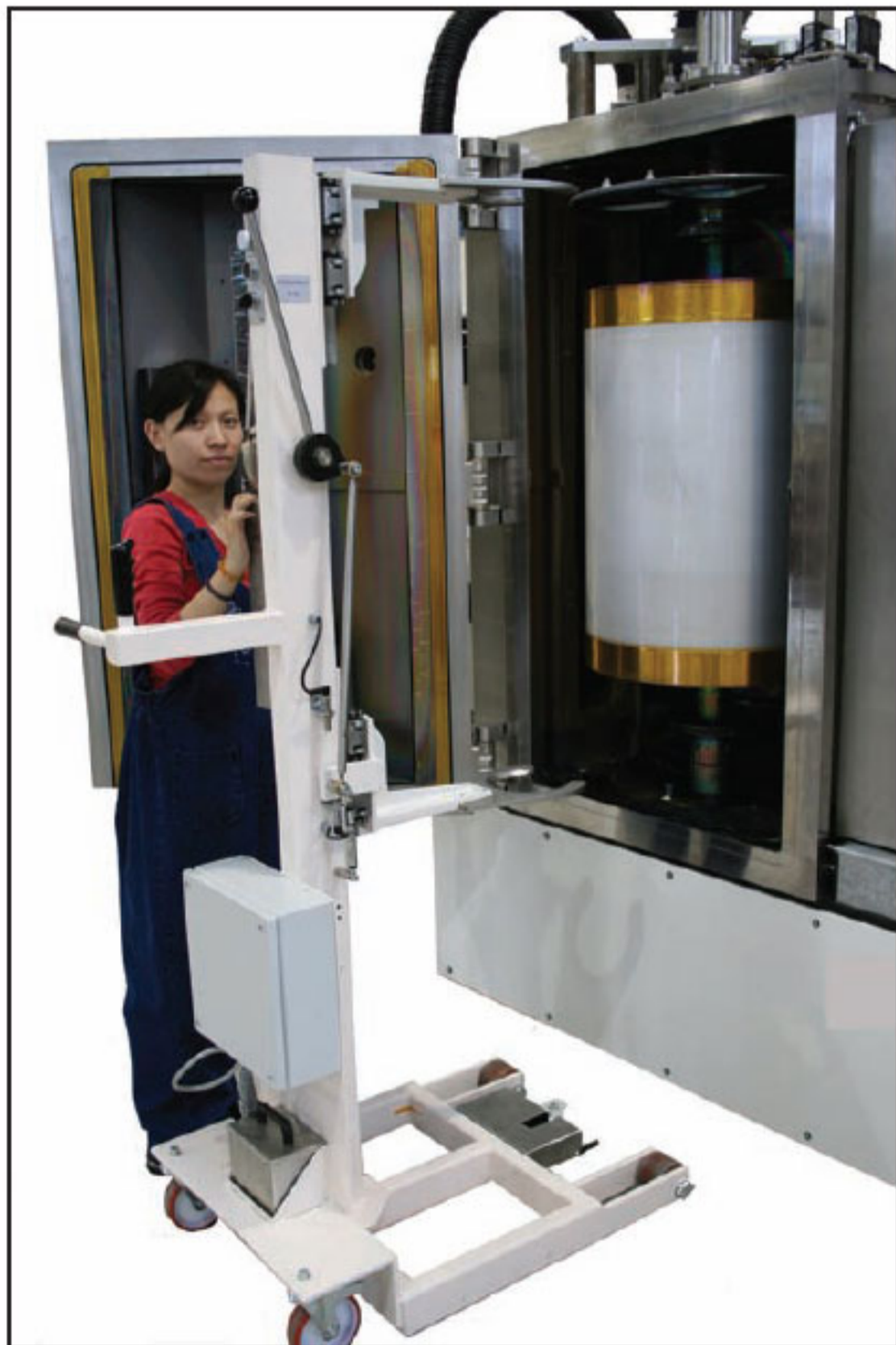
Figure 1. The CFM850 system uses a 0.5-m retractable cylindrical drum for substrates and 1-m linear magnetrons for deposition. In this case, the machine is being used to deposit a six-layer high-performance antireflection coating on a 1.4 \times 0.6 -m polycarbonate sheet.
