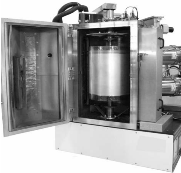
Figure 2a. CFM850 coating system from Applied Multilayers Ltd. The system is also fitted with a rotating shutter to expose the substrate to the appropriate target. The shutter is also used to enable targets to be conditioned without exposure to the substrates.
