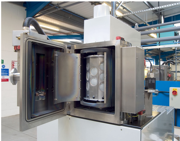
Figure 2a CFM450 AR coating system from Applied Multilayers Ltd.
